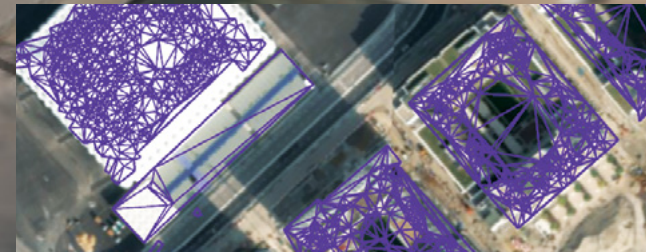
Automatic Feature Extraction (AFE) of buildings from a 0.5m, Next Generation Automatic Terrain Extraction (NGATE) DSM. Imagery courtesy of Ordnance Survey Great Britain.
